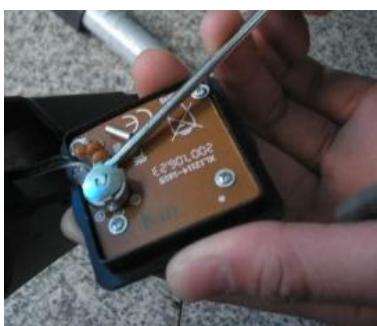
Using a small screwdriver, replace the battery (LR44) and set the control unit back in the housing. Place the LCD-unit in the front again and press it into the frame until it clicks into place.
