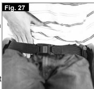
Generally the Lap Belt should be fixed so that the straps sit at an angle of approximately 45°, and when correctly adjusted should not allow user to slip down in the seat. (Fig. 28)
